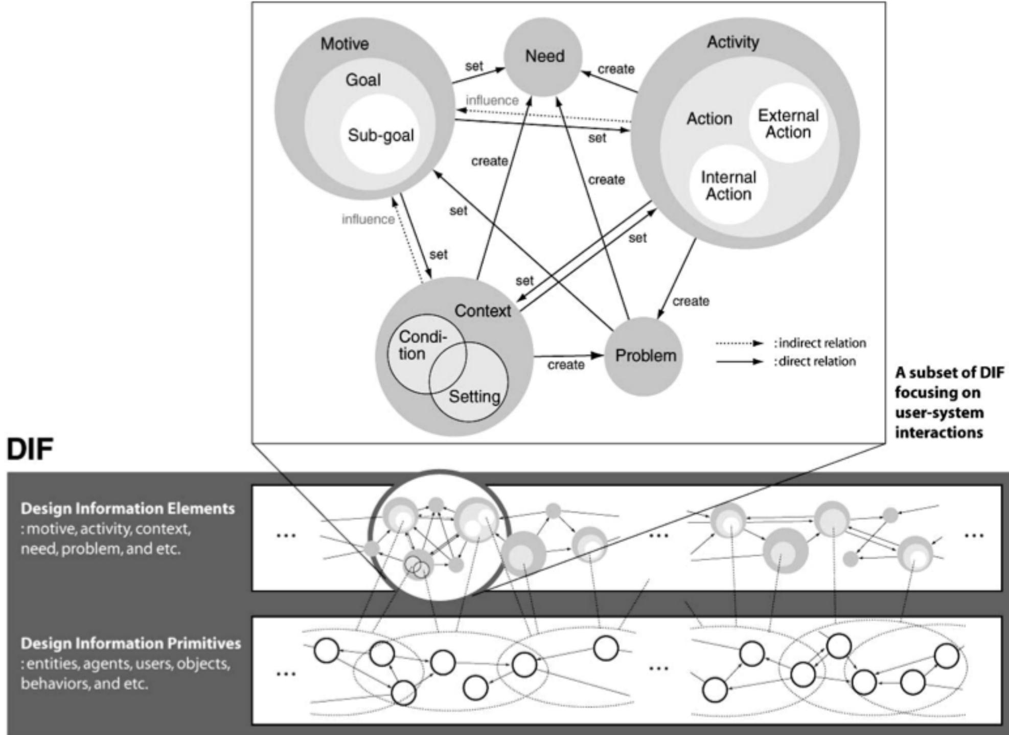
Figure 2 Relationship between the elements and the primitives of design information in DIF
