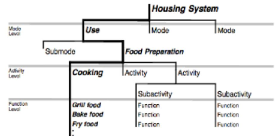
A three-level, top-down analysis is used to find Functions that cover the requirements of a system. The result is a Function Structure.
